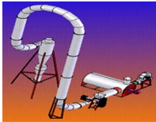
Technical Sketch of the Flash Dryer
